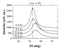
Fig. 2.  $\theta$ -2 $\theta$  X-ray diffraction scans for several  $[Fe(t)/Cu(3t)]_8$  superlattices with different Fe layer thickness. Dashed lines indicate the calculated spacings for a superlattice with  $\alpha$ -Fe  $(d_{110}(\alpha$ -Fe) = 2.02 Å) and a superlattice with ferromagnetic  $\gamma$ -Fe  $(d_{111}(\alpha$ -Fe) = 2.102 Å).
