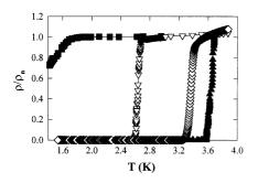
Fig. 3. Resistivity vs. temperature curves for several  $[Fe(t)/Cu(42 \text{ Å})]_8/200 \text{ Å}$  Nb multilayers: filled squares, t = 5 Å; hollow triangles t = 7 Å; filled triangles, t = 11 Å; hollow rhomboids, t = 20 Å. Each curve has been normalized by the normal state value of the resistivity  $\rho_n$  just above the transition.
